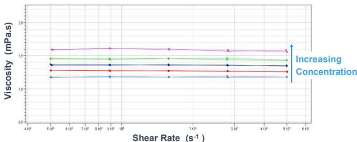
Figure 2: Viscosity of HEC LR 250 solutions at different shear rates.
