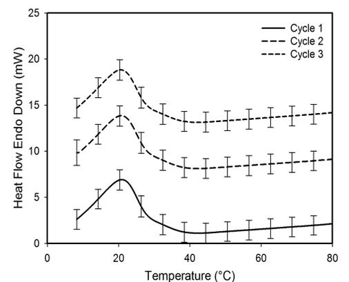
Figure 3- MicroDSC Thermograms of Cooling Cycle
