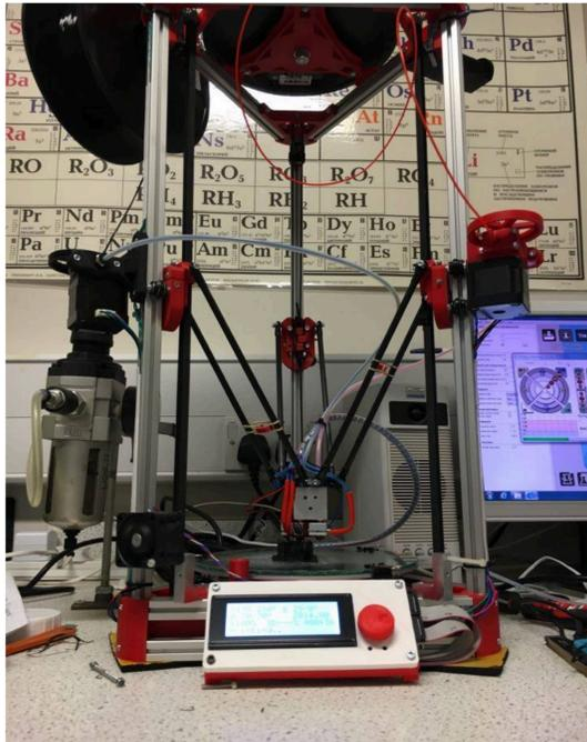
Figure 1- FDM Printer
