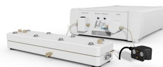
The experiments were performed on an HPLC consisting of an isocratic pump, an auto sampler and a variable wavelength detector coupled to a Wyatt DAWN HELEOS II MALS detector and a Wyatt Eclipse AF4 (with center downstream injection technique, together with a custom-made EAF4 channel)
