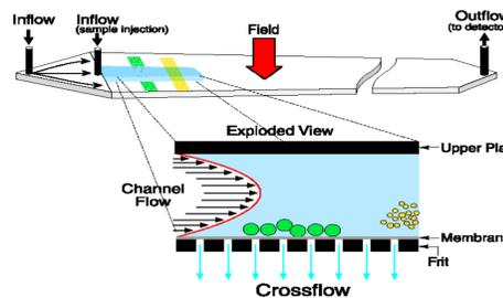
Modified design introducing a variable electric field as a modifier on sample behaviour and separation
